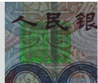
■ IR 740 - 1100 nm illumination for «Anti-stokes inks» examination
